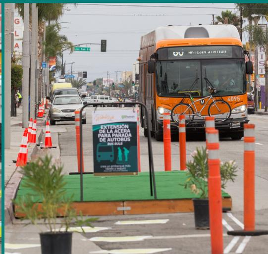
**3** Bus bulbs align the bus stop with the parking lane decreasing the amount of time lost when merging into and out of traffic improving boarding efficiency.
